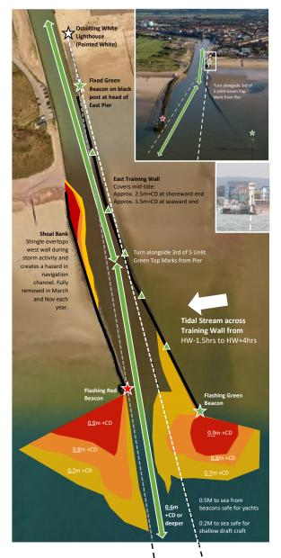
Additional Transit Helpful at Lower Tides Lighthouse (Occulting White) and Drumhead Pile (Quick Red) 352° / 173 ° Standard Approach Transit on Charts Lighthouse (Occulting White) and East Pier Head (<u>Fixed</u> Green light/ small black post on SE corner of Pier) 346° / 166°
