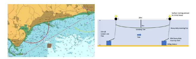
Two Kelp Farming Lines will be deployed a maximum of 20 meters apart with mooring configuration as pictured. Seeded lines (which the kelp grows on) will be suspended downwards of 6m below the waterline. The extents of the farm will be marked by 4x spherical Special Marks (lit with sequence FI.Y.5s) each with X topmarks. The farm will be located within the 0.5 NM by 0.5 NM area licensed by the MMO marked in orange on the chartlet above.
